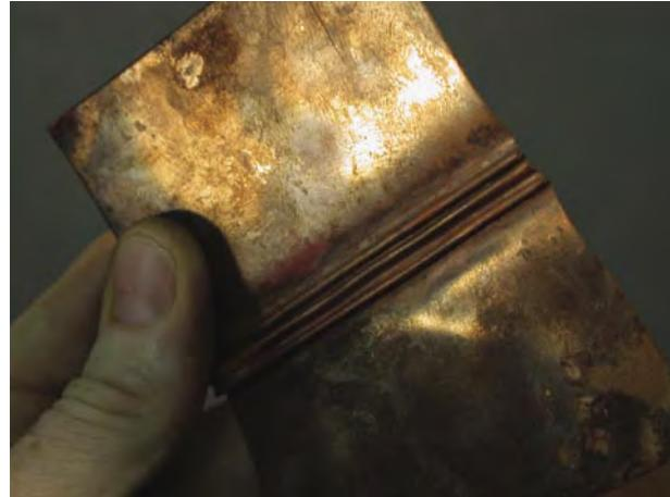
4. When annealed and unfolded, confirm the lines by pressing them down with a planishing hammer or rolling mill. This will make the lines crisp, as with the basic line-fold. The process can be repeated to make multiple sets of lines across a sheet.
