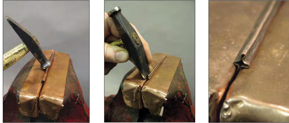
3. Drive the sides of the loop in with a hammer or a chasing tool to create the cross shape. This is a miniature version of the process shown on the preceding page.
